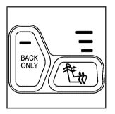
Your vehicle may have heated front seats. The buttons used to control this feature are located on the front door armrests. The engine must be running for the heated seat feature to work.
